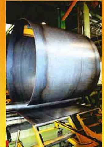
Tankrolling in progress
